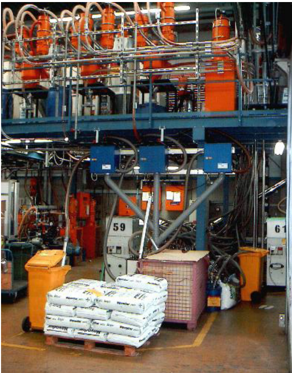
Three MESEP Extraktor 70 provide for metal-free products.
